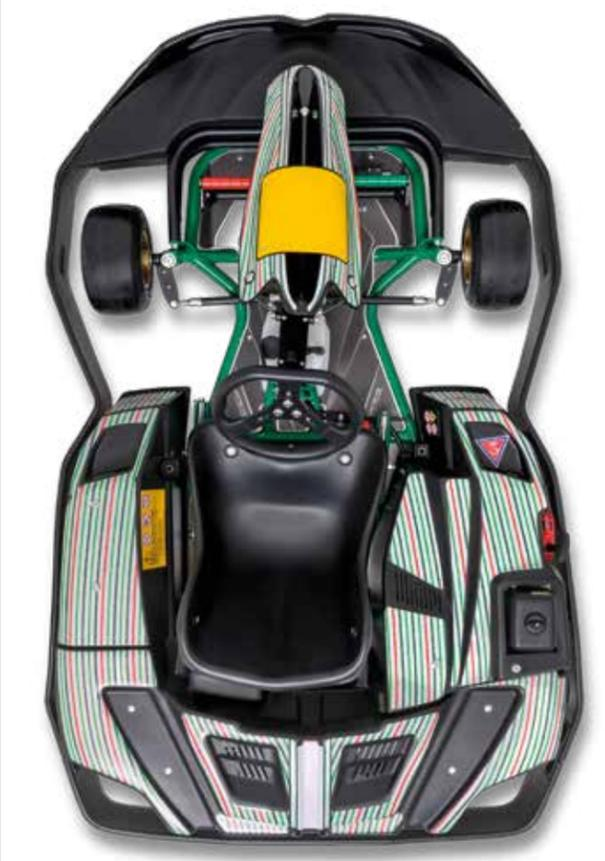
The junior rental kart shares all of the impact protection systems which are found thoroughly tested on the adult rental kart. This can be seen with the protective plastic perimeter band around the chassis protecting the driver as well as the chassis and steering components. Large polyurethane shock absorbers positioned in specific areas on the chassis also prevents the driver or kart from any damage.
