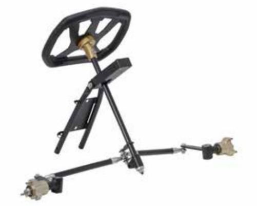
The cushioned steering column, with its guaranteed 5cm controlled movement, allows energy to be dissipated in the event of a collision, thereby safeguarding the drivers upper limbs
